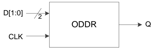
Figure 3-13 I/O Logic in DDR Output Mode
