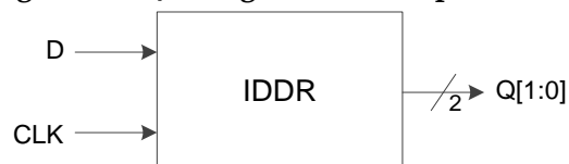
Figure 3-12 I/O Logic in DDR Input Mode
