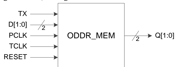
Figure 3-23 I/O Logic in ODDR_MEM Mode
