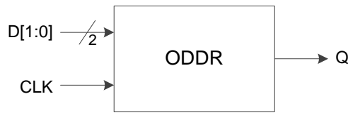
Figure 3-19 I/O Logic in DDR Output Mode
