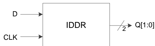
Figure 3-18 I/O Logic in DDR Input Mode
